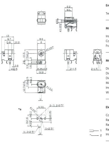
\*a printed circuit board layout, solder side view
