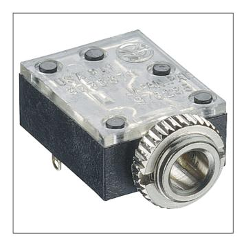
Jack chassis socket acc. to JIS C 6560 JC35J3B, 3.5 mm, 3 poles/stereo, angular version, with 2 break contacts and solder eyes, for printed circuit boards, for back side mounting
